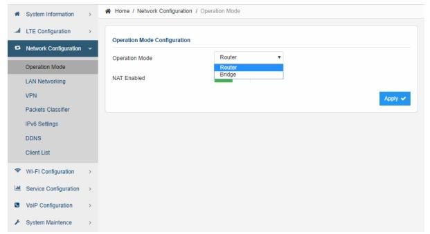
The device operation mode could be changed from Router to Bridge if necessary as show by the following diagram:
