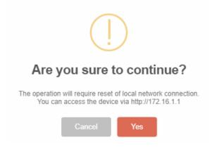
In Bridge mode, the PC which connected the LAN port of the CPE will obtain the IP directly from the network. However, the device WEB GUI may still be accessed via port 8080 from remote side if remote management is enabled. For local LAN access, the user or operator can configure LAN PC with a static IP address as 172.16.1.x and login the WEB GUI via http://172.16.1.1.
